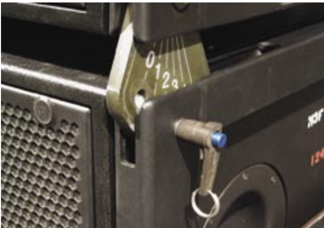
Figure 20. QRP inserted at 3°
